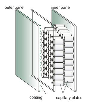
The 2-pane make-up consists of one 20 mm cavity with two 10 mm capillary slabs and covering pane, in general without coating.
