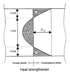
technically-cooled glass. The temperature resistance is also much higher than normal glass. In the following comparison of some of the technical data the most important differences between plate glass (float glass), heat strengthened glass based on float glass and tempered glass according to DIN 1249 "Flat glass in civil engineering" Parts 10 and 12 "Tempered glass".
